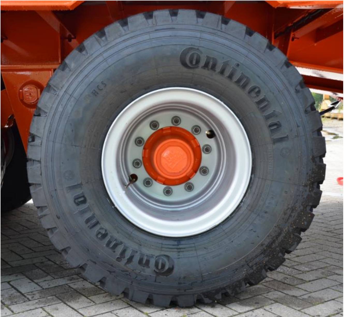
Example: 10" rim (10 holes) with 14.00 R 20 tire
