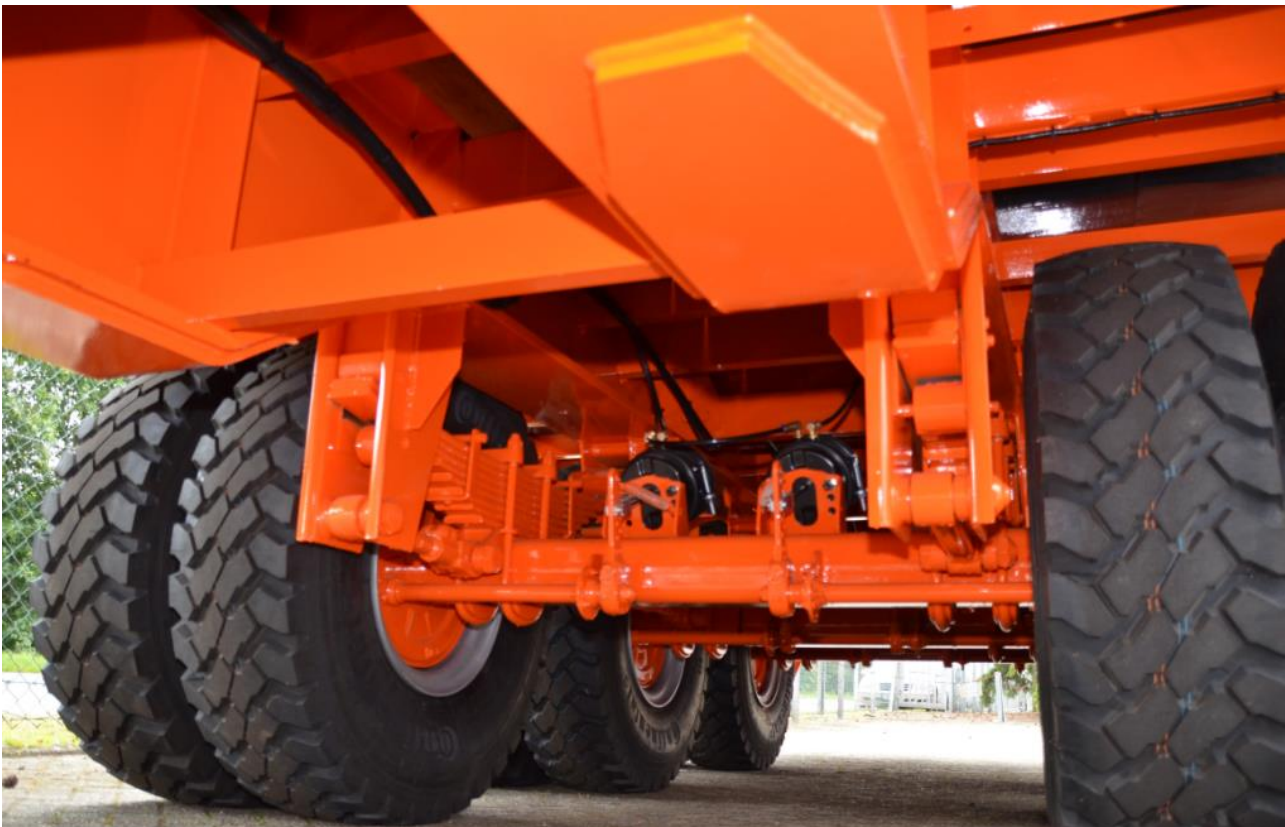
Axles: BPW – Mode: VBT 3/18010 - Capacity 18 to. each. Off-Road Tires: 14.00 R 20
