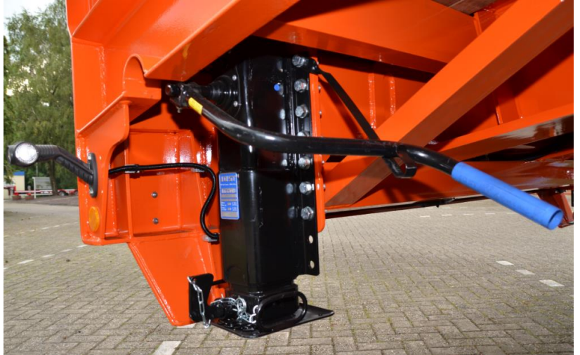
Heavy duty rear support of hydraulic ramps (Landing Gears). They are manually operated, one-side operation . Please notice the strong protection of the landing gear on the trailer chassis.
