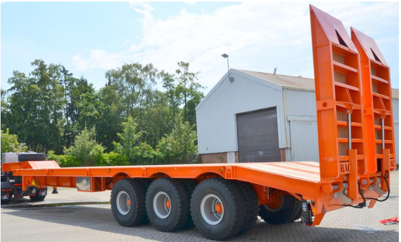
Heavy duty off-road low bed semi-trailer for the safe transportation of construction machines
