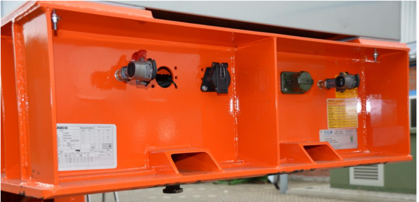
Very well protected connection ports (air and electricity) against all kind of damages.
