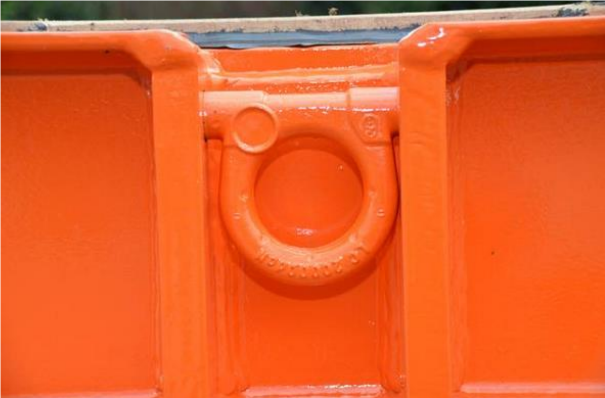
Load security: 5 pairs heavy-duty lashing eyes, 20 ton each, welded along each trailer side.
