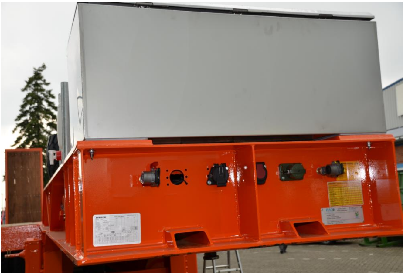
On top of the gooseneck the metal tools and equipment box (lockable).
