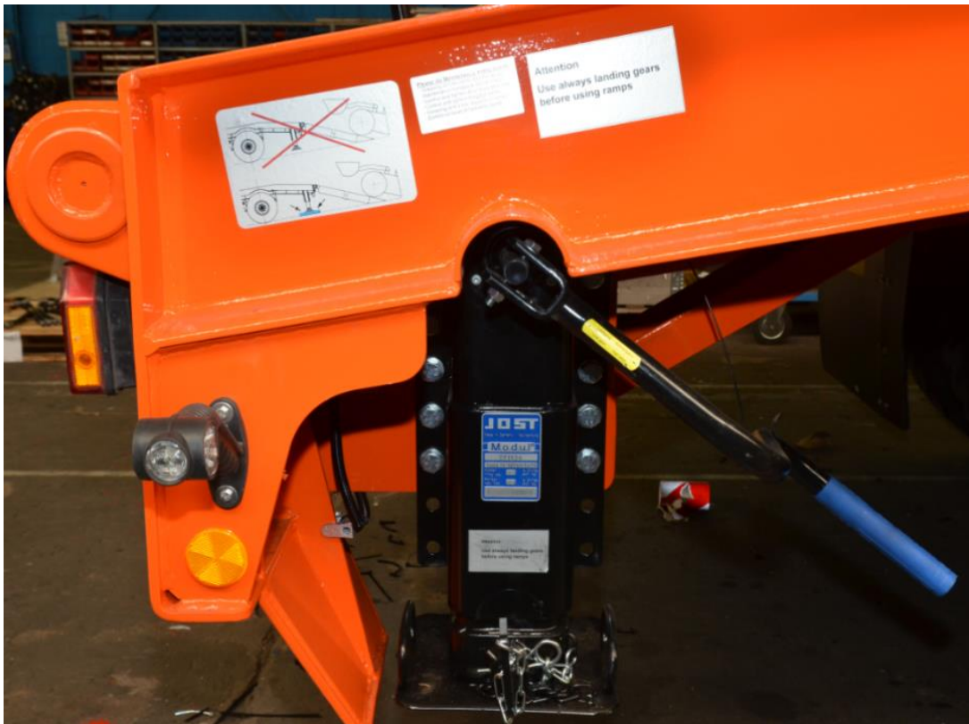
Please notice the strong rear protection of the landing gear
