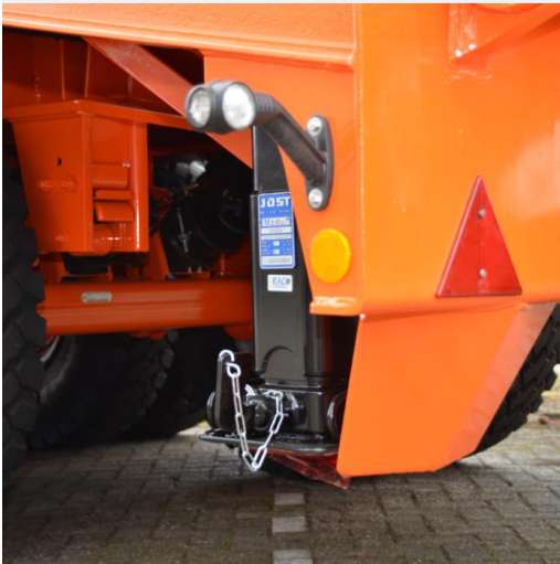
Heavy duty rear support of hydraulic ramps (Landing Gears). They are manually operated, one-side operation . Please notice the strong protection of the landing gear on the trailer chassis.
