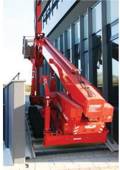
The outriggers and automatic levelling system allow the operator to set the Spider up on different levels. This is needed as the Spider is being set up on the steps of the grandstand. The easy-to-use controls with colour coded functions also make the Teupen Leo 36T very user-friendly.
